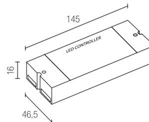
Control unit model SR-1029 for Single color, CCT or RGB LEDs with three radio frequency remote controls.
