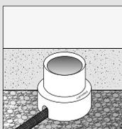
*Install outer casing placing upper part flush with the floor. Apply equipped cap in order to avoid entry of foreign bodies on recessed box. Provide an appropriate drainage under the outer casing.*
