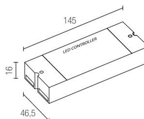
*Control unit model 1029W for RGBW LEDs with radio frequency remote controls.*
