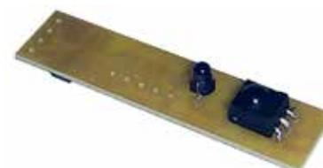
*The electronic device is designed to turn the LEDs on and off thanks to a Infrared Sensor. It is necessary to approach the Sensor at a distance of 10 cm to switch the LEDs on or off. Wired with 50 cm in/out.*
