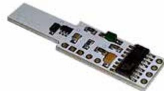
*The electronic device is designed to dimmer and turn the LEDs on and off thanks to a Touch Sensor. Wired with 50 cm in/out.*
