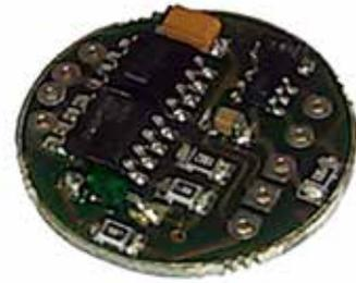
*The electronic device is designed to turn the LEDs on and off thanks to a Touch Sensor. Wired with 50 cm in/out.*
